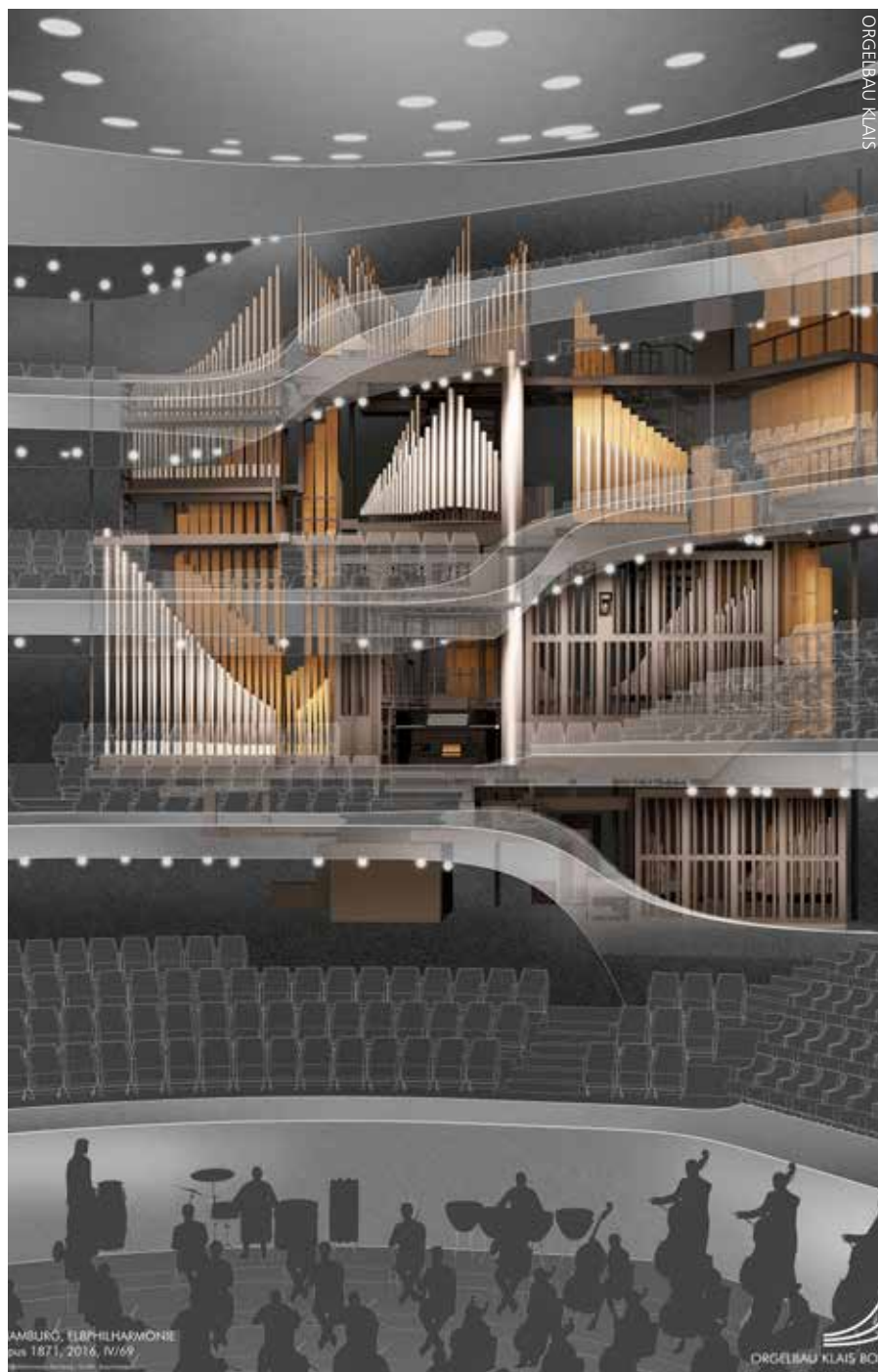
THIS GRAPHIC OF THE NEW ORGAN IN THE ELBPHILHARMONIE IN HAMBURG, GERMANY, SHOWS HOW SOME OF THE 4765 PIPES ARE DISTRIBUTED NEXT TO AND BEHIND THE TERRACED ROWS OF SEATS.
